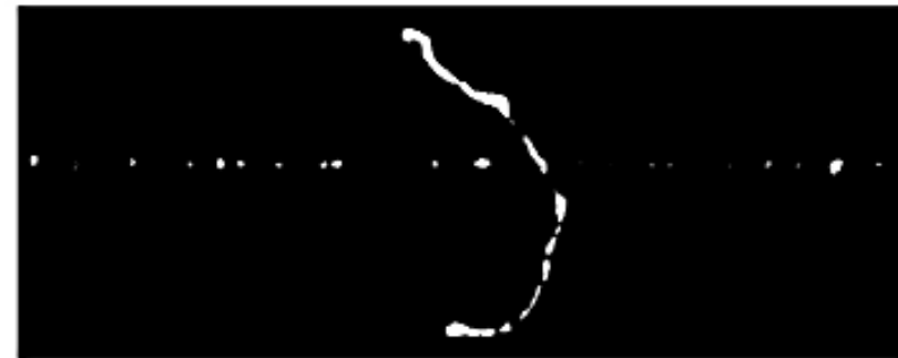
(c) Cloud chamber tracks of a fast electron (circa 200kV) crossed by a dense track from a slow electron (circa 20kV); at this low energy the track is bent because of scattering.
